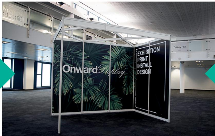
Panels slot into shell scheme system. Poles exposed every 1m creating 40mm gap between panels.
